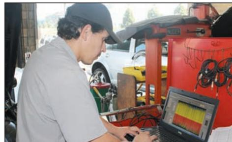
Technician Carlos Herrera uses the shop's PC-based scan tool to diagnose a rough-running engine problem.
